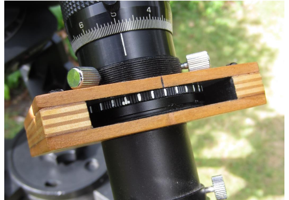
The polariser has marks every 10 degrees
