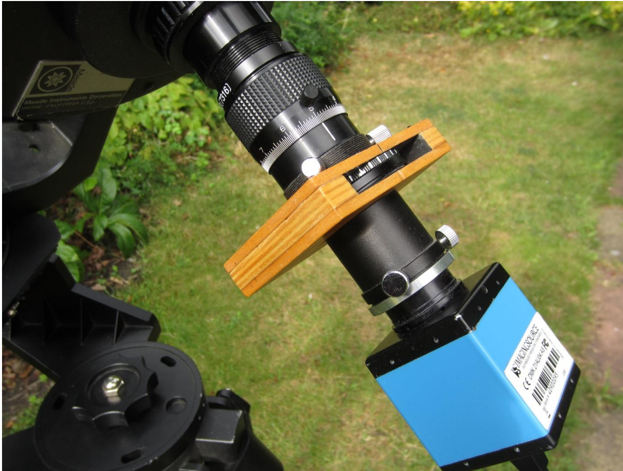
Rotating polariser mount attached to 20 cm Meade LX-10 SCT
